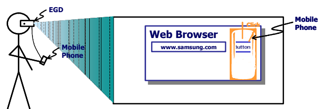
Figure 1. The concept of mobile pointing & input system.
