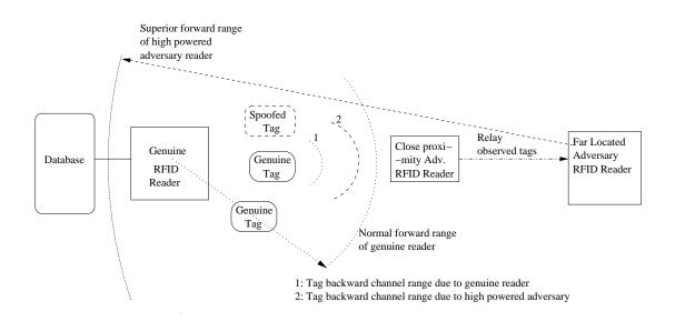
FIG. 3.1. A threat model showing spoofed tags and collaboration between adversary readers located at different distances
