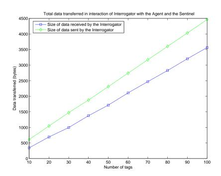
FIG. 7.18. Total data transfer in interactions of the Interrogator with the Authenticating Agent and the Sentinel
