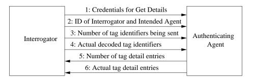
FIG. 7.6. Interrogator gets the details of the respective tags from the Authenticating Agent
