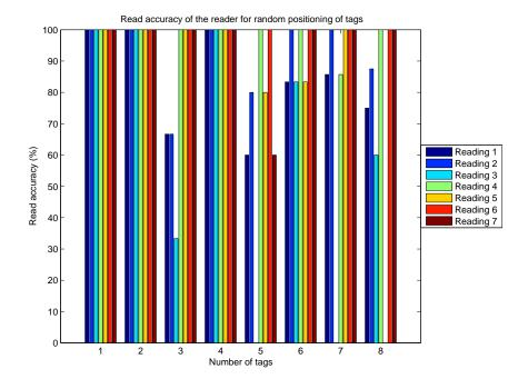
FIG. 7.9. Reader read accuracy for random positioning of tags
