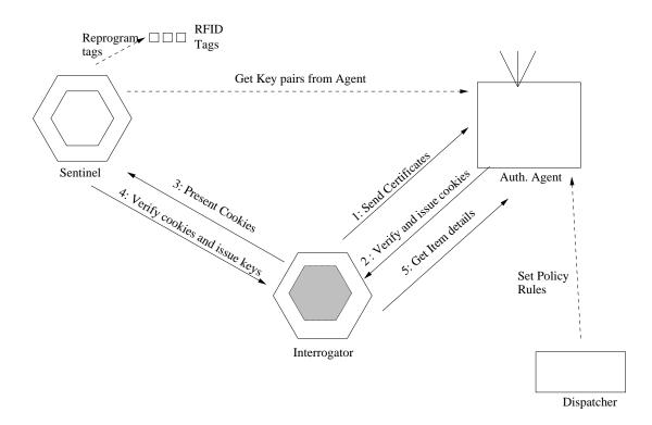
FIG. 6.2. Interrogator communication with the Authenticating Agent and Sentinel to learn the tag identifiers
