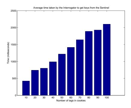
FIG. 7.13. Time taken by Sentinel to issue decoding keys to Interrogator
