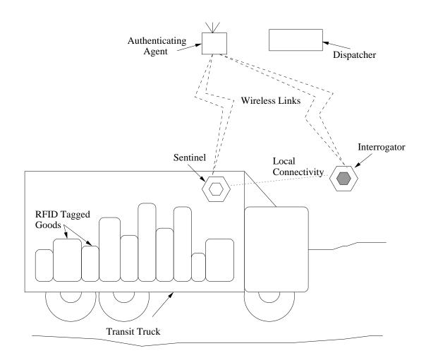
FIG. 6.1. Authenticating. Agent and Sentinel collaborate to give an authorized Interrogator access to tag identifiers
