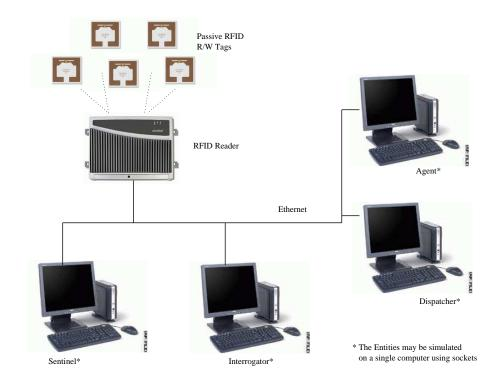
FIG. 7.1. Our prototype consists of a RFID reader connected to a computer system
