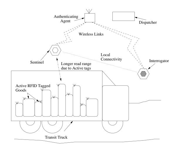
FIG. 6.3. In an approach using active tags, the tags have a longer communication range and have wireless connectivity
