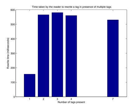
FIG. 7.10. Time taken by reader to rewrite to a specific tag in presence of a number of tags
