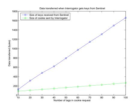
FIG. 7.14. Data transfer involved in an Interrogator getting decoding keys from the Sentinel
