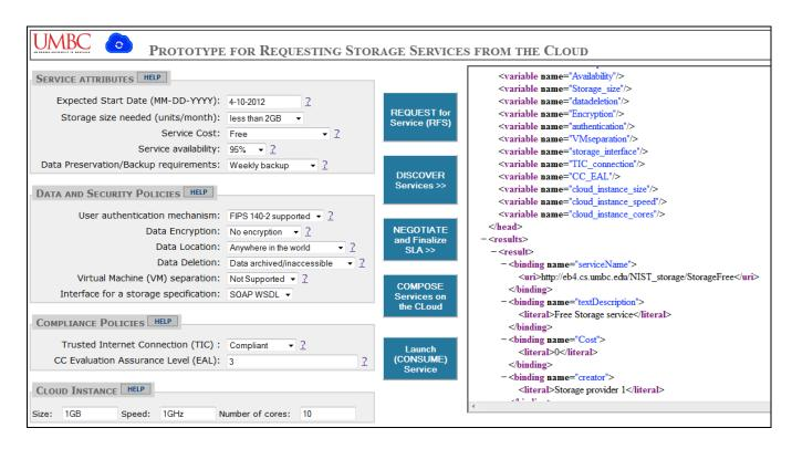
Figure 4: Matching Services are returned along with service IRI and constraint value.
