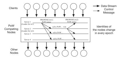
Fig. 4. The message flow for PoW-based blockchains. Control messages are the messages for nodes to compete for PoW.
