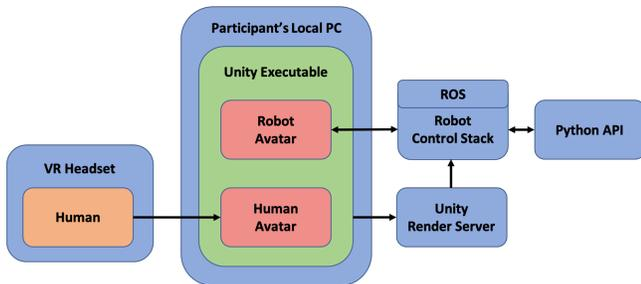
Figure 2: A high-level architecture of the RIVR system
