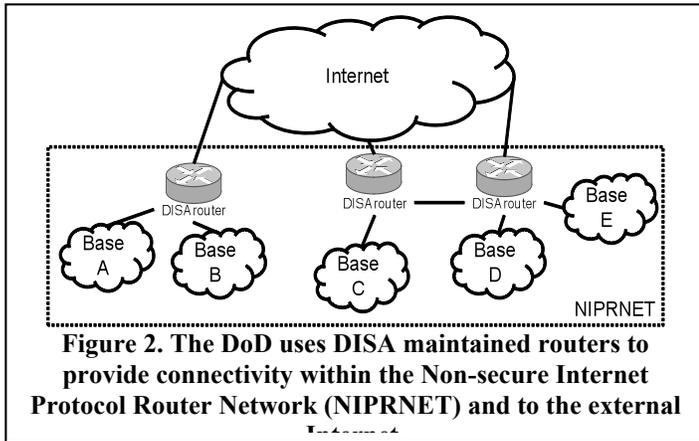
**Figure 2. The DoD uses DISA maintained routers to provide connectivity within the Non-secure Internet Protocol Router Network (NIPRNET) and to the external**
