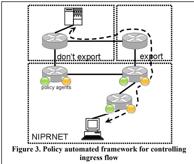
**Figure 3. Policy automated framework for controlling ingress flow**
