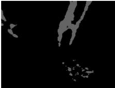
Fig. 5.1 Image obtained after thresholding hue channel
